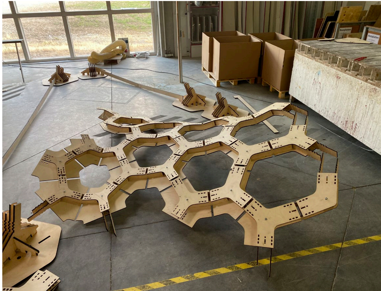
Test assembly of two segments
